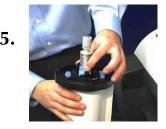
5. Replace Left Paper Flange and lock by pressing down the Blue Lock Tab
