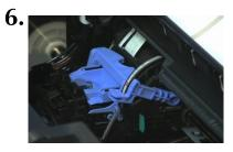
6. Close Blue Plastic Covers on Print Head Shuttle and close top machine cover.
